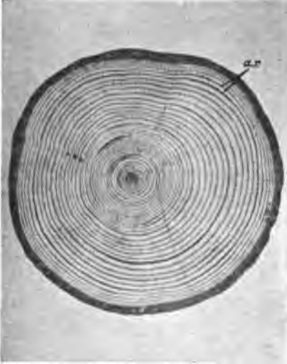
FIG. 8. — Transverse Section of the Stem of a Young Balsam Fir Tree, Showing Annual Rings of Growth, a.r. , \frac{1}{2} Natural Size. (Bull. 55, U. S. For. Ser.)
